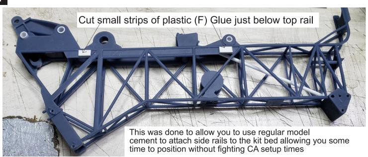
Build your Frame and bed according to the Plastic kit Instructions For the Tamiya kit. In Step 7 do not use the spare tire. Step 18 Jerry Can Rack
